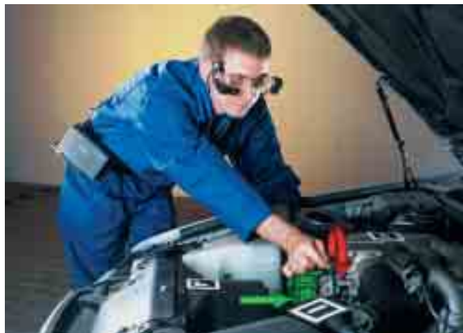
Figure 1: Augmented Reality manual for service task with a wearable computer
